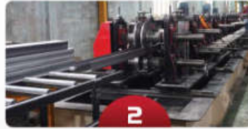
2 Quy trình cắt, cán rail, cán rung Cutting process, rail rolling, vibration rolling
